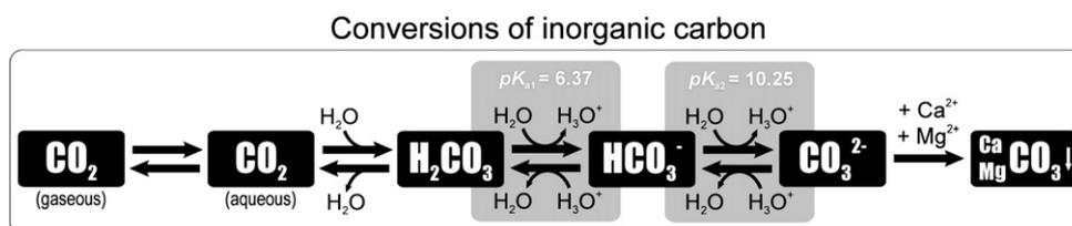
Fig. 1. Conversion of inorganic carbon species including acid–base ionization/dissociation constant ( $pK_a$ ) values for the hydrogen carbonate (bicarbonate) anion. See text for further details.
